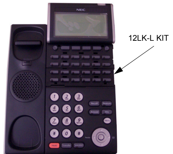
Figure 7-25 Installing the 12LK-L KIT
