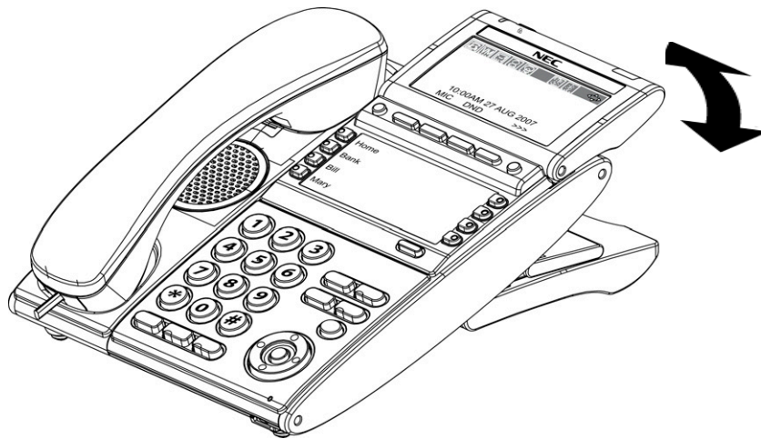
Figure 7-20 Adjusting the LCD on a Multiline Terminal
