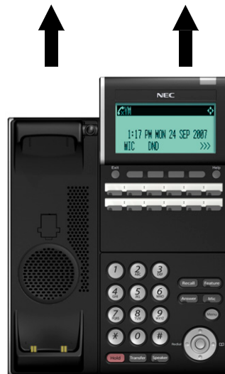
Figure 7-47 Removing the Multiline Terminal
