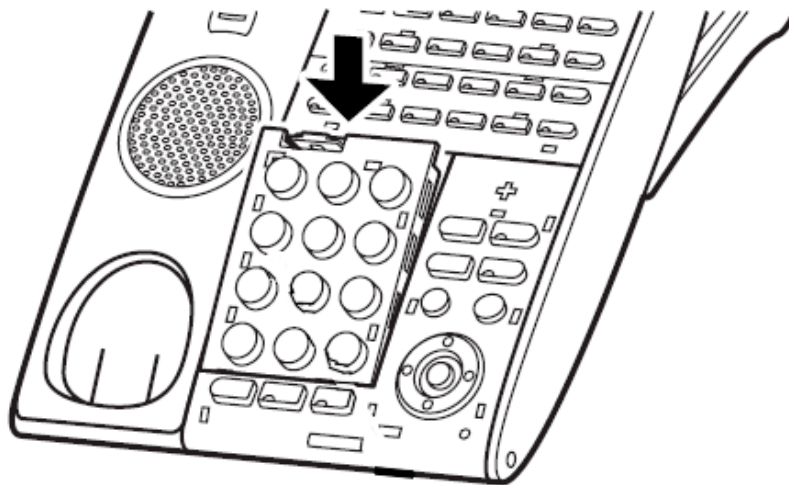
Figure 11-70 Install Numbered Keypad
