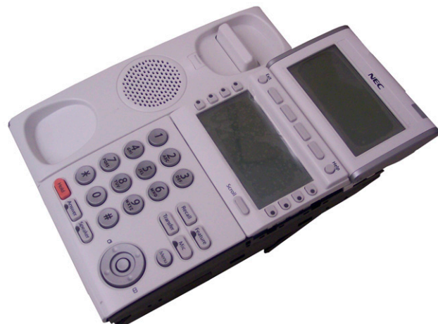
Figure 7-58 8LKD (LD)-L UNIT Installed
