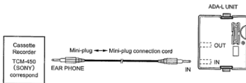
Figure 11-53 ADA-L IN Jack Connection
