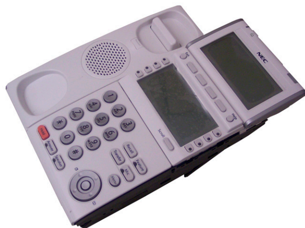
Figure 7-64 8LKI (LD)-L UNIT Installed
