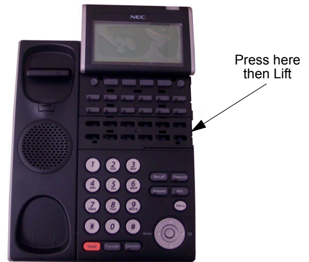
Figure 7-24 Removing the Line Key Placeholder
