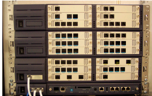
Single CHS1U-US Rack Mount with Three CHS2U-US Expansion Chassis
