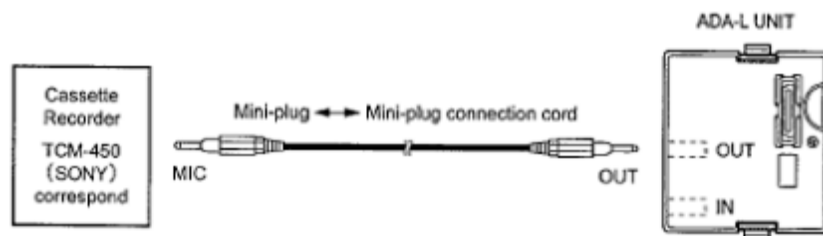
Figure 11-52 ADA-L OUT Jack Connection
