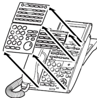
Figure 11-68 Remove Plastic Panels
