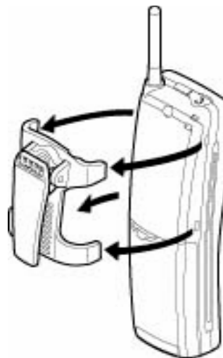
Figure 8-21 Removing the Belt Clip
