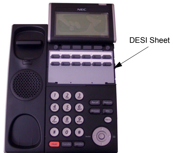
Figure 7-23 Removing the DESI Sheet
