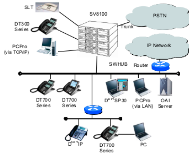
Figure 1-1 Simplified SV8100 System Connectivity
